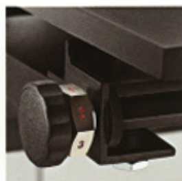
Rotary knob for setting the programme shaft for the hole centres
